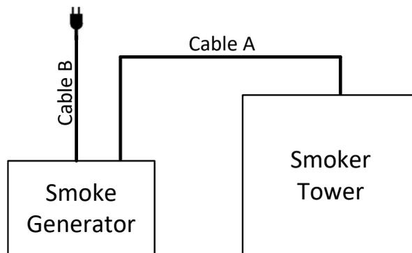
Figure 3.1 Power Cable wiring for Original Bradley Smoker
